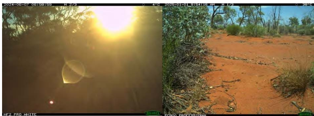
Figure 25 left- Camera 49B facing east causing overexposure and false detections early in the morning and right, 49A field of view significantly obstructed.
